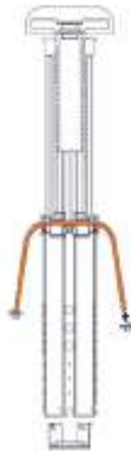
Attach plug to free end of band, securing band in place.
