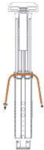
Slide inner tube up and out until channel is visible, threading the new band through the outer tube with plug on one end.
